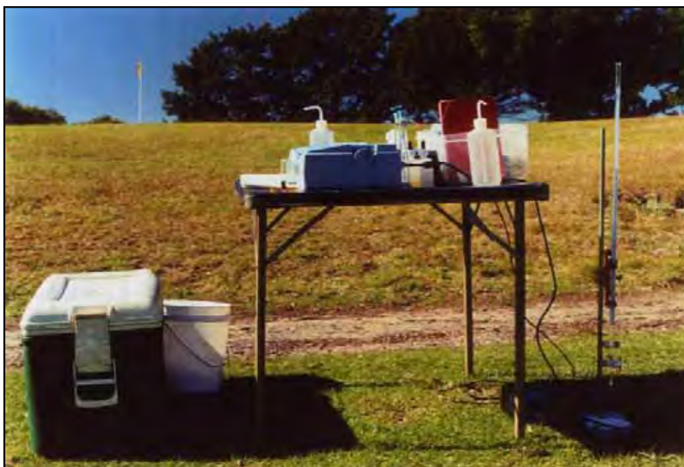
Figure 5.8 Field equipment for analysis of redox sensitive elements.
