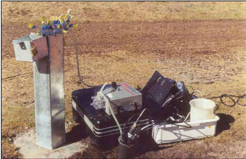
Figure 5.7 Purging sample point and measurement of field water quality parameters.
